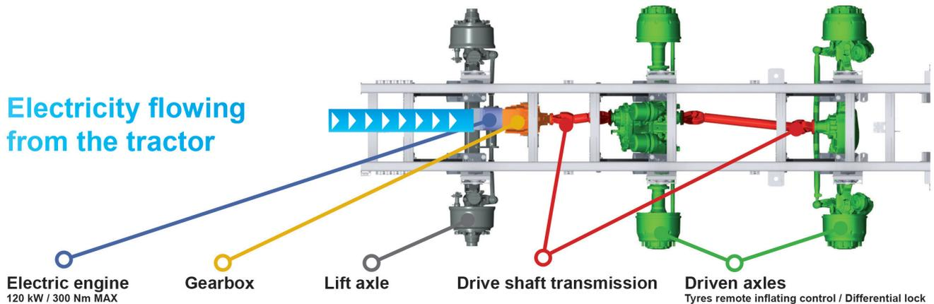
JOSKIN's E-Drive technique is a hybrid system based on many key elements, the most important of which is the motor. Real main piece of the system, this engine of the SCHABMÜLLER manufacturer transforms the received electric energy into a mechanical power up to 120 kW at a 210 Nm couple (max. 300 Nm). The clutch transmission box is provided and designed by DINTEC.
