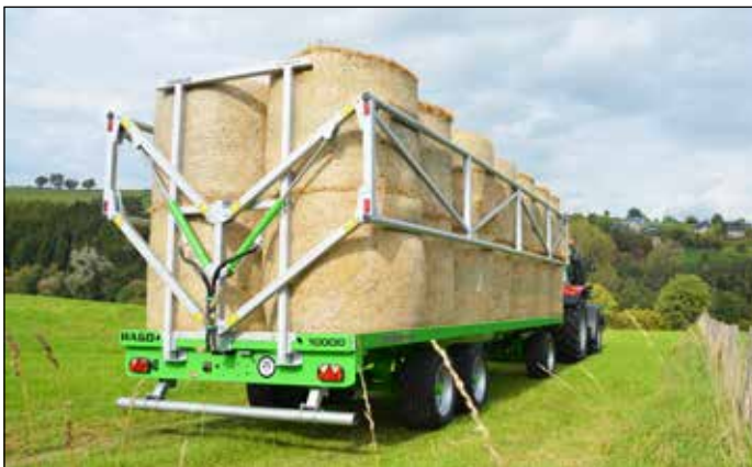
Lifting and lowering by means of hydraulic ram
