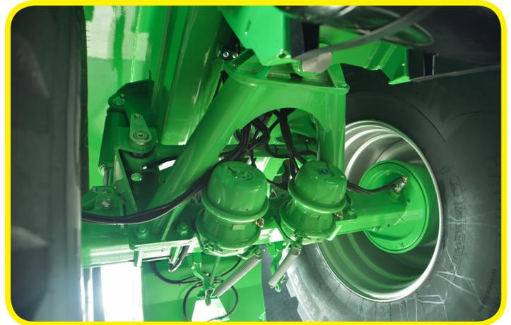
articulated triangular structure. Already successfully used on dump tipping trailers, this suspension type allows to better follow the ground, whatever its topography, as well as a higher maintenance ease (lubrication, etc.).
