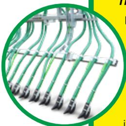
**The *Pendislide Basic*** will be rather used to fertilize meadows. This spreading boom is fitted with wear-resistant Ertalon skids applying a continuous pressure on the ground by means of a system of spring leaves. By moving apart the vegetation, these skids ensure a precise distribution of the nutrients close to the roots without dirtying the leaves or fodder.
