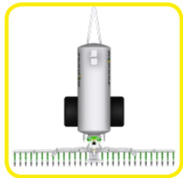
easily on a Ø 600 mm manhole. The 2 fixing arms are directly bolted on the tanker bracket. In this way, these 2 new models can easily be mounted on new and existing tankers without having to add extra pieces of equipment. They are also compatible with the ALPINA2 and MODULO2 models if the wheel diameter is lower than 1,820 mm. If there is a linkage on the tanker, these booms are also compatible.
